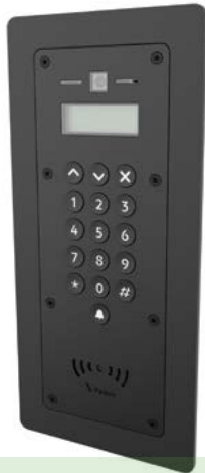
The Entry panel is a robust door entry panel incorporating both door entry and access control functions. It is powered using power over Ethernet (PoE) and communicates with the other elements of the system using IPv6, providing 'plug and play' installation. Each panel is associated with a Entry control unit which is the interface to the door hardware.
