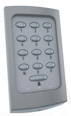
The KP75 MIFARE® keypad reader is a RFID/Keypad combinations device that offers the convenience of contactless authentication, or the added security of PIN/Prox entry, for system users.
