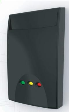
Our Proximity energy saving reader minimises energy wastage and saves customers money on their utility bills. The reader cover is designed to retain a user card. Once inserted, the card's presence in the reader toggles a relay that switches on all connected equipment. When the card is removed, the relay toggles back, turning all equipment off.
